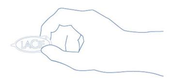
2. Insert the pointed end of the drive lock tool into the E-boot port on the back of the device. You will feel minor resistance as you push the reset button.
