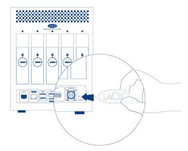
3. While you are pushing the reset button with the drive lock tool, turn on the LaCie 5big NAS Pro by pushing the front LED button. DO NOT remove the drive lock tool as the LaCie 5big NAS Pro powers on. Doing so will prevent the LaCie 5big NAS Pro from using the LaCie USB Key as the boot device.
