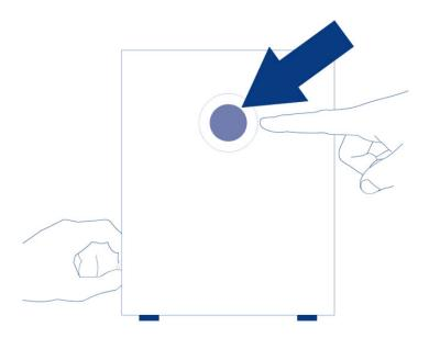
4. Release the reset button 10 seconds after all the rear disk LEDs turn solid blue.
