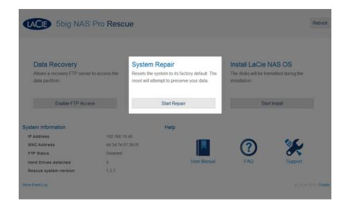
• Install LaCie NAS OS: The Rescue will format the LaCie 5big NAS Pro hard drives before reinstalling LaCie NAS OS. Since all data will be deleted during the format, LaCie highly recommends that you back up your files before selecting this option.
