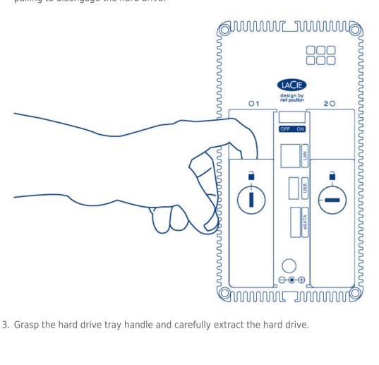
3. Grasp the hard drive tray handle and carefully extract the hard drive.
