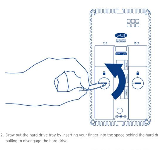
2. Draw out the hard drive tray by inserting your finger into the space behind the hard drive tray handle and pulling to disengage the hard drive.
