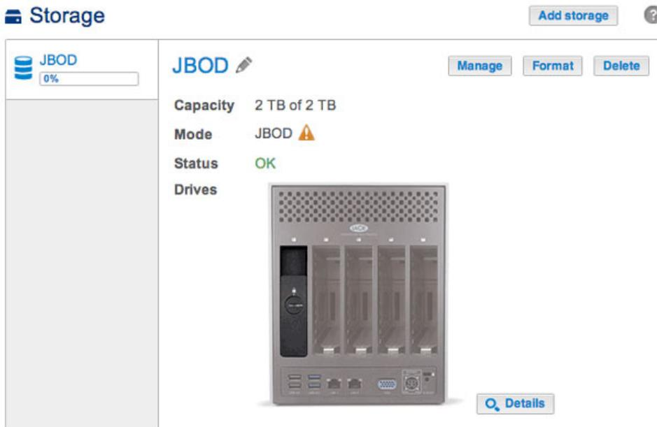
The screenshot above shows a single-disk volume configured for JBOD (for instructions on how to change the name of the volume from the default to *JBOD*, see [Volume Tools](#)). Follow the steps below to add one or more drives to your JBOD volume: A JBOD volume can be expanded with new disks added to the LaCie 5big NAS Pro enclosure.
