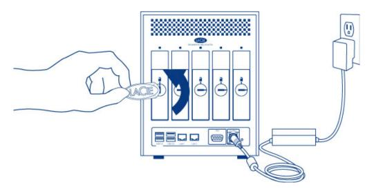
2. Draw out the hard drive tray by inserting your finger into the space behind the tray handle and pulling to disengage the tray.
