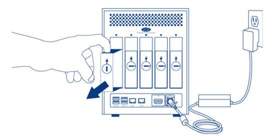
4. To reuse the disk tray, unfasten the drive's screws and affix the new disk to the tray. Detailed instructions are available at <u>Connect to the Network: Diskless LaCie 5big NAS Pro</u>.
