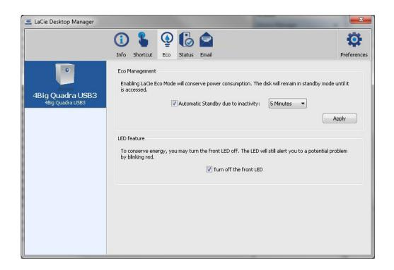
By default, your drive will enter Eco Mode after **5 minutes** of inactivity in order to conserve energy. To exit Eco Mode, simply access data and the disks will automatically restart, or click the product's front button.
