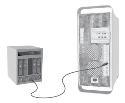
**Technical note:** If two interfaces are connected at the same time, the first one connected remains active and the second will not work.
