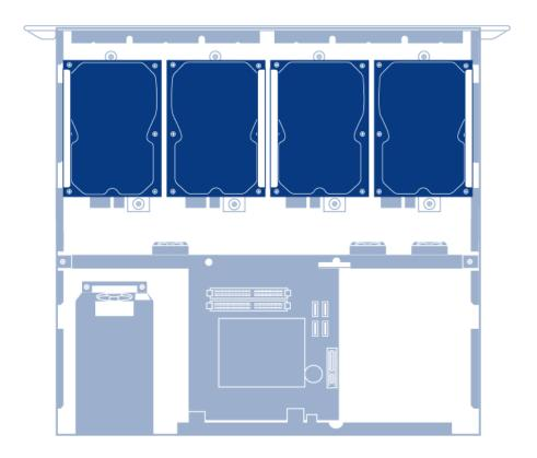
The 4big contains two drive frames, each housing two 3.5-inch form factor disk drives. The frame has mounting locations for SATA drives. The drive frame provides thermal conduction, radio frequency, and electro-magnetic induction protection and affords the drive physical protection.
