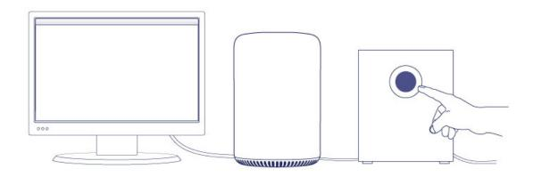
Apply a short press to the front LED button to power on the LaCie 5big.
