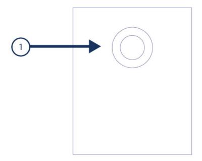
1. **Status LED/power button:** The LED indicates that the device is powered on and provides status signals (see <u>System LEDs</u>). It is also the power button. A short push will spin down the LaCie 5big's hard drives and place the system into idle mode. A long push is for emergency use only since it cuts power to the system without spinning the hard drives down. See <u>Operation</u> for more details.
