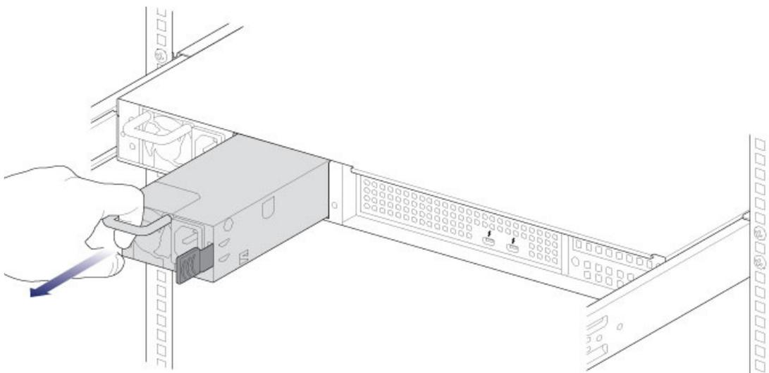
4. Insert the replacement PSU into the empty PSU slot.
