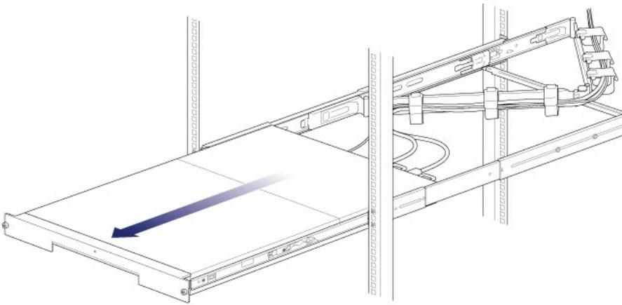
3. Release the cover by simultaneously pushing both front latches toward you.
