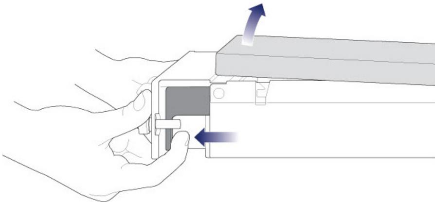
4. Lift the cover and remove it from the enclosure.
