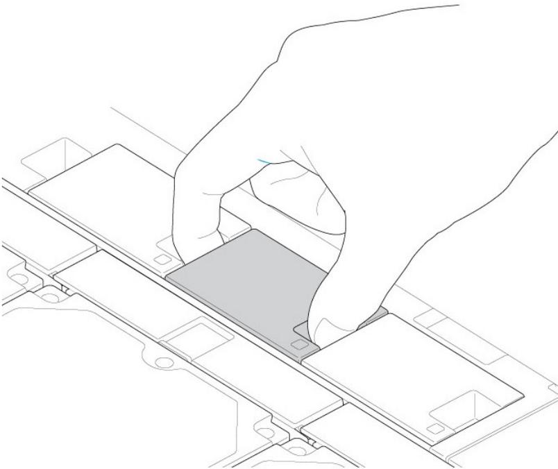
3. Lift the fan from its slot. **Show caution when removing the fan since moving parts can cause severe damage.** The fan should stop rotating once it is removed from its slot.
