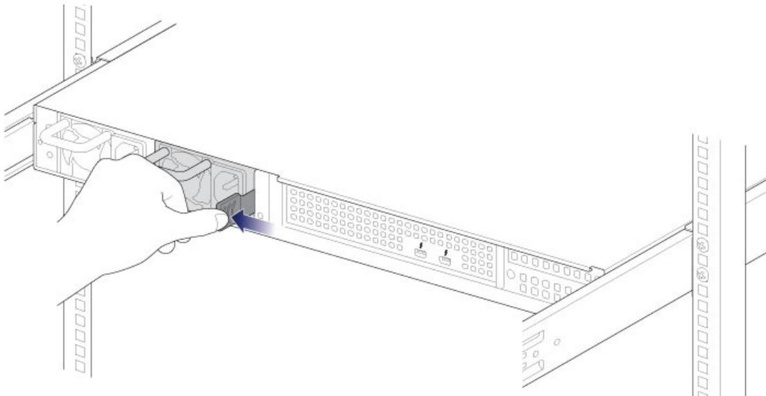
3. Remove the PSU by pulling the handle away from the LaCie 8big.
