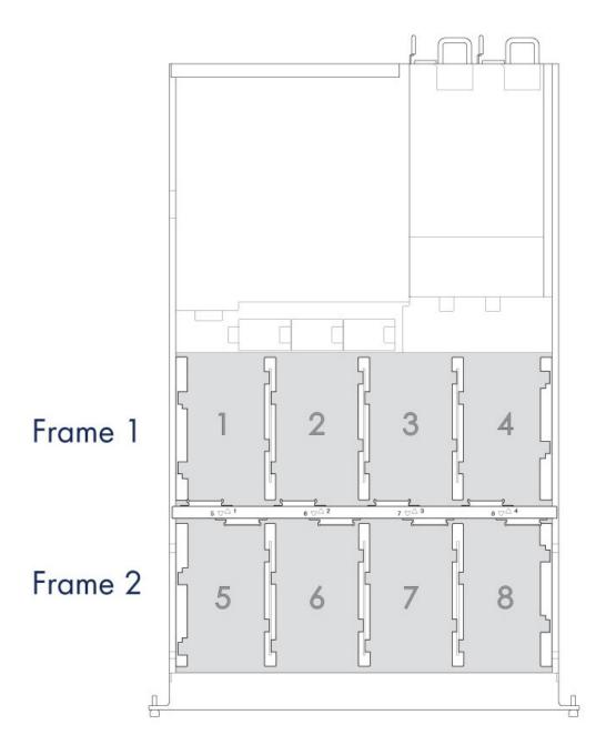
The LaCie 8big Rack Thunderbolt 2 has two hard drive frames, each housing four 3.5-inch hard drives. Each frame has mounting locations for SATA connections.
