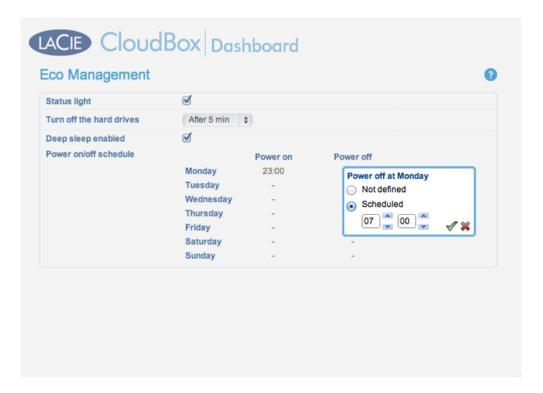
**Power on:** The device wakes from deep sleep mode. **Power off:** The device enters deep sleep mode.
