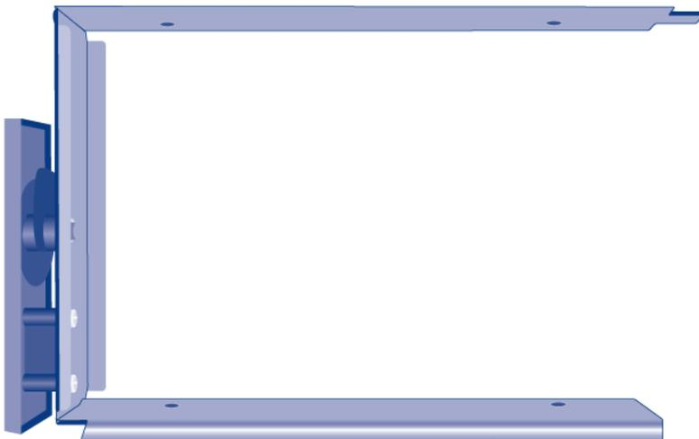
2. Many disks have a label on one side and the printed circuit board on the opposite side. With its label side facing up, gently place the hard disk within the drive tray. Keep the side with the printed circuit board on the work space and the SATA connector facing to the right. The four tray screw slots should align with the disk's four screw holes.
