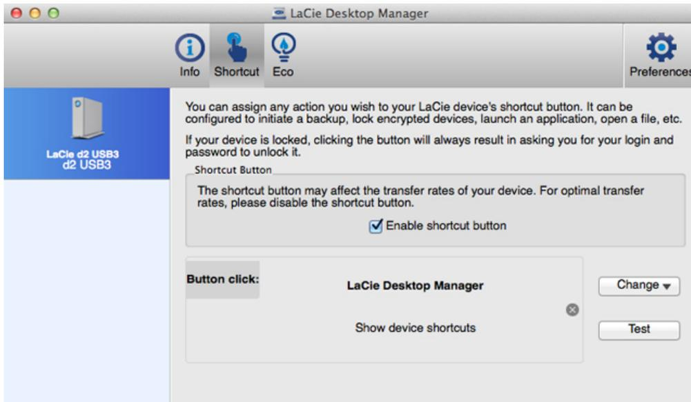
Configure a short press of the LED button to launch an application. A short press is one second. The default setting for the Shortcut is LaCie Desktop Manager but you can browse for your preferred application. For example, set the LED button Shortcut to launch your operating system's photo application.
