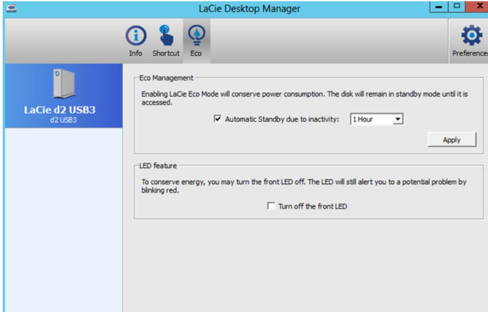
Set the time that the LaCie d2 is inactive before entering Eco mode. Eco mode is also known as power-saving mode.
