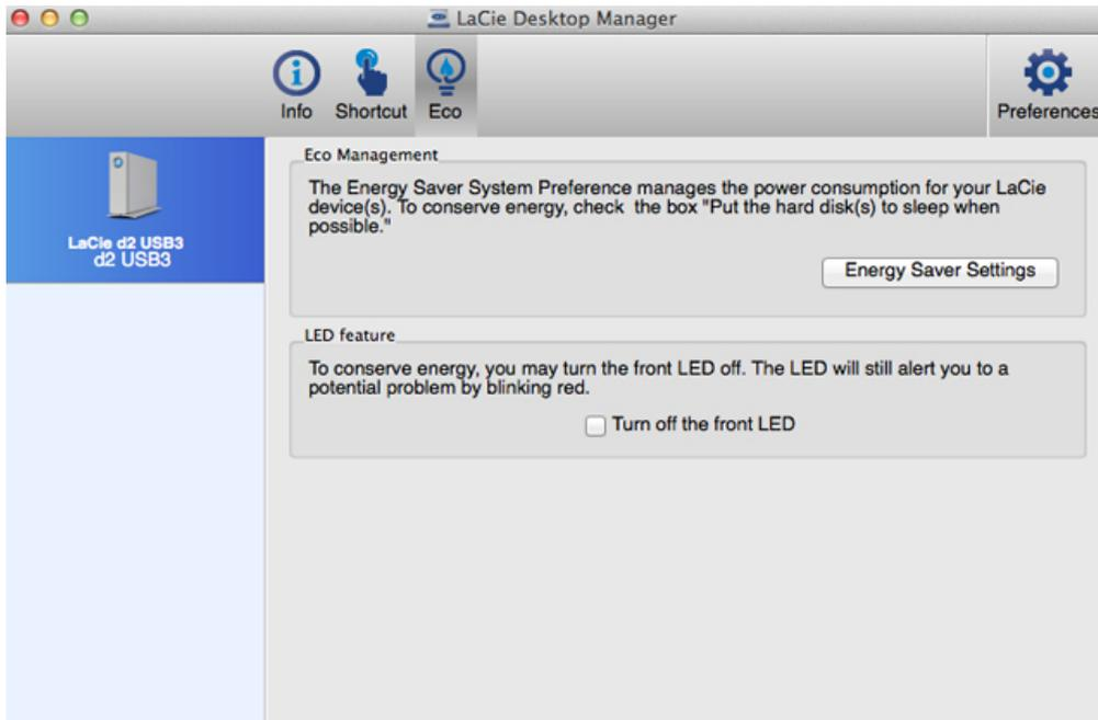
The Mac OS manages the power-saving mode for external devices. Choose **Energy Saver Settings** in LaCie Desktop Manager to launch the System Preferences. Within the Energy Saver preference, select the option to put external hard drives to sleep when possible.
