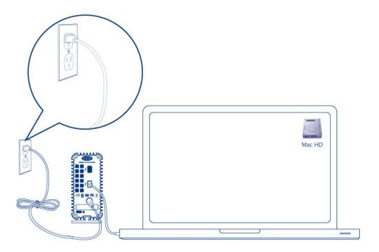
3. The device will turn on automatically and the volume will mount on the desktop.
