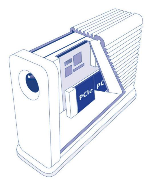
At the heart of the Little Big Disk Thunderbolt 2 are two PCle Gen 2 SSDs. The use of PCle Gen 2 SSDs place the Little Big Disk Thunderbolt 2 into the next level of advanced storage. Most standard multi-disk enclosures that feature SSDs or HDDs share a SATA bus. No matter the version of SATA, the drives are limited to a fixed number of channels to pass data. However, each PCle Gen 2 SSD has its own bus which helps to limit data bottlenecks from multiple drives.
