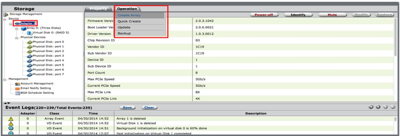
3. Add hard drives on the Create New Array page. To select a hard drive, click on its icon. A check mark appears next to a selected hard drive.
