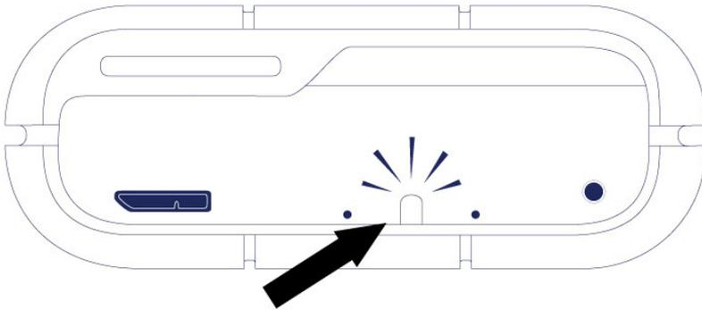
Use a thin, pointed object to push the RAID select and RAID confirm buttons. For example, use the pointed end of a paperclip to access and push the buttons.
