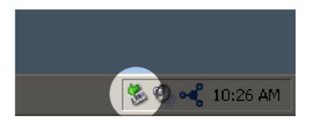
This message will appear: "Safe to Remove Hardware" (or similar). It is now safe to disconnect the device.
