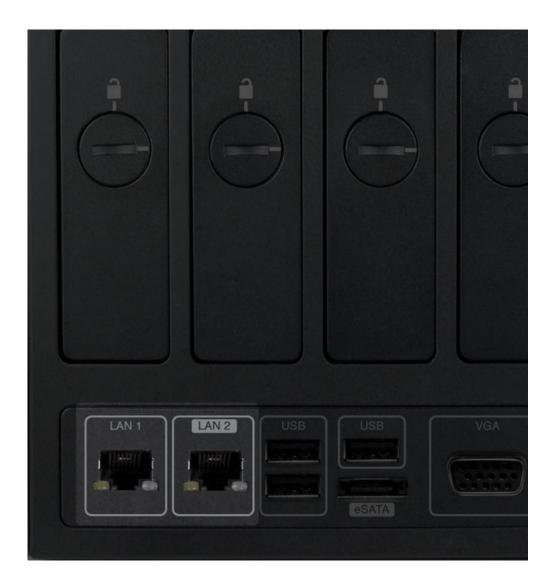
Most connections to a network use a single Ethernet port on a computer, server, or network device. However, you may set the LaCie professional server for Ethernet Teaming by attaching a second Ethernet cable and configuring the included Intel® driver.
