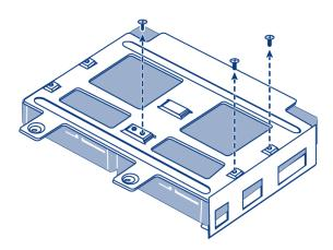
8. Screw in the four screws securing the drive frame to the chassis.
