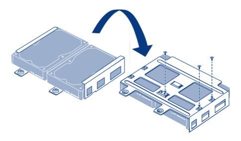
6. Turn the drive frame over again, then slide the hard drive out from the hard drive frame, and slide a new one in. Make sure that the large printed label on the hard drive is pointing up.
