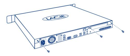
3. To remove the cover, slide and lift at the same time.
