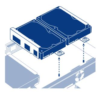
5. Turn the drive frame over. While supporting the drive with one hand, remove the three screws securing the drive to the drive frame.
