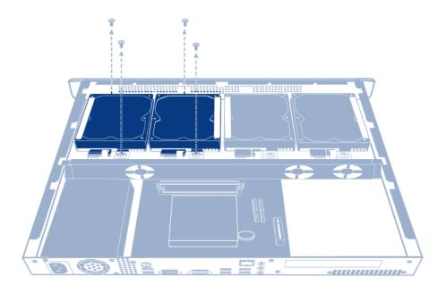
4. Lift the drive frame out of the chassis.
