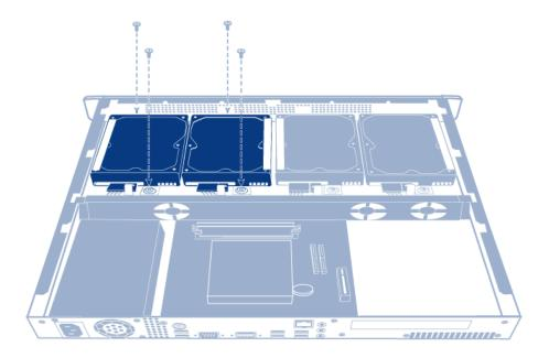
9. Reconnect the SATA and power cables. Be careful to ensure that the numbers correspond to the correct disk number (from 0-3). The cables and disks are numbered to make this easier.
