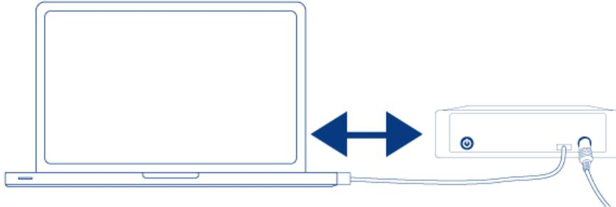
**Important info regarding the interfaces:** Only one interface type may be used to connect your computer to the device. Unmount the drive from your computer if wish to switch between the USB 2.0 and FireWire 400 interfaces.
