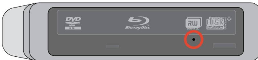
4. Insert a small metal poker, such as the end of a paper clip, into the emergency eject hole until it presses against the manual eject mechanism. You will feel the mechanism eject the disc tray.
